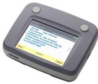
A lightweight, battery powered reader with color graphical touchscreen display.
